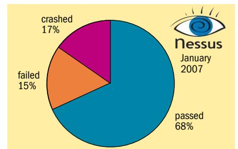
*Results of vulnerability tests performed by CERN on PLCs using standard penetration tools.*
